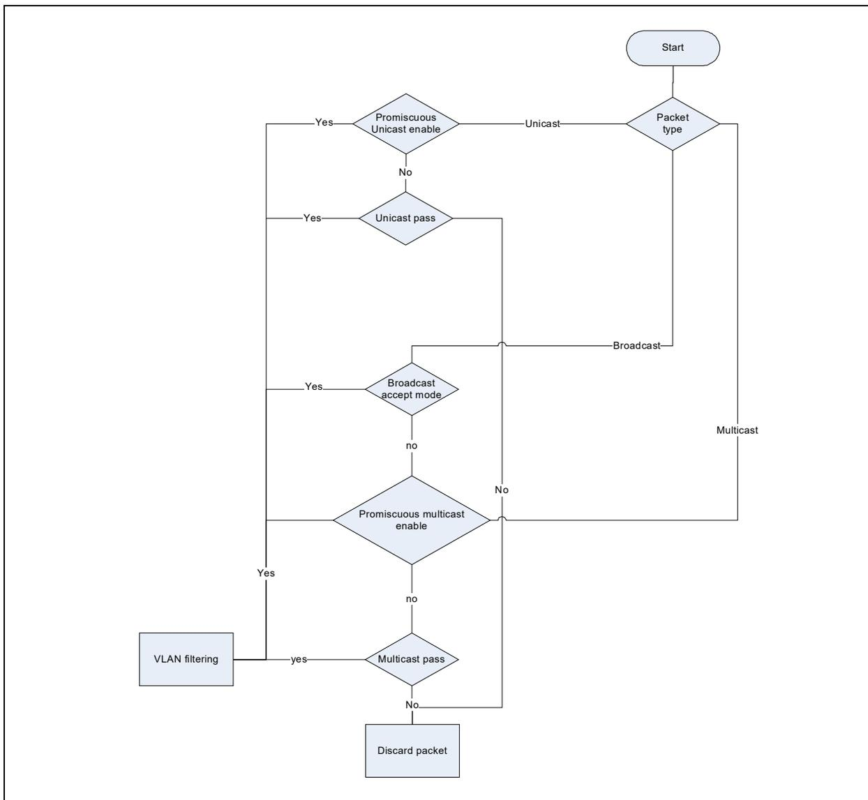
Figure 7-2. Host MAC Address Receive Filtering Flow Chart
