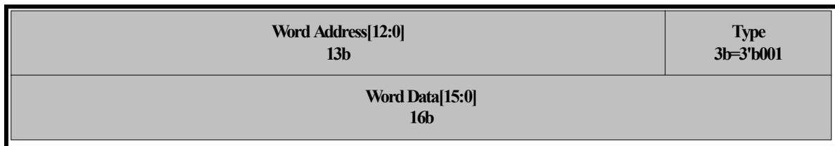
**Figure 6-1. Shadow RAM Word Write Command**
