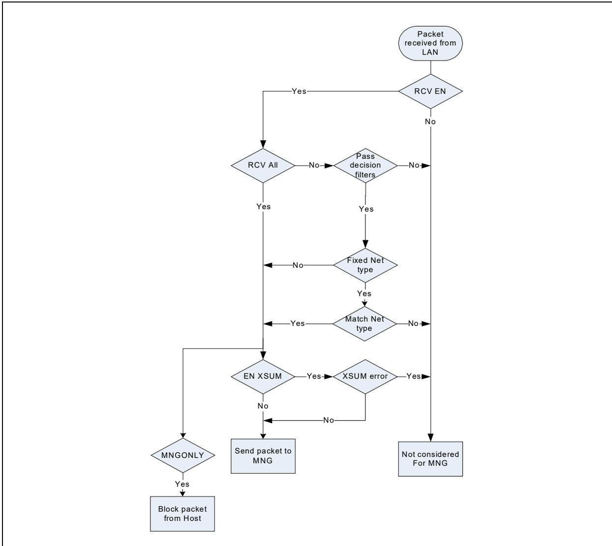
Figure 7-4. Manageability Filtering
