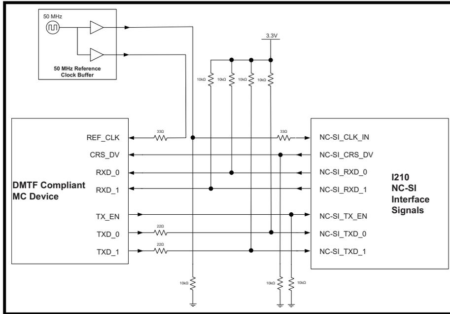
Figure 12-17. NC-SI Connection Requirements - Single-Drop Configuration
