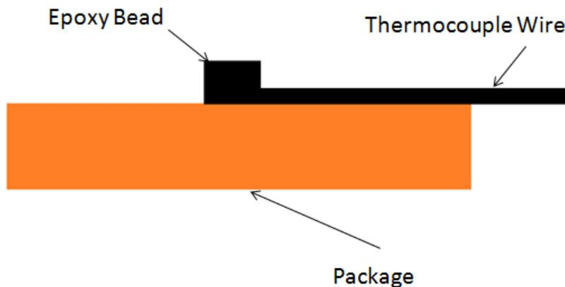
**Figure 13-29. Technique for Measuring  $T_{\text{case}}$  with  $0^\circ$  Angle Attachment, No Heat Sink**
