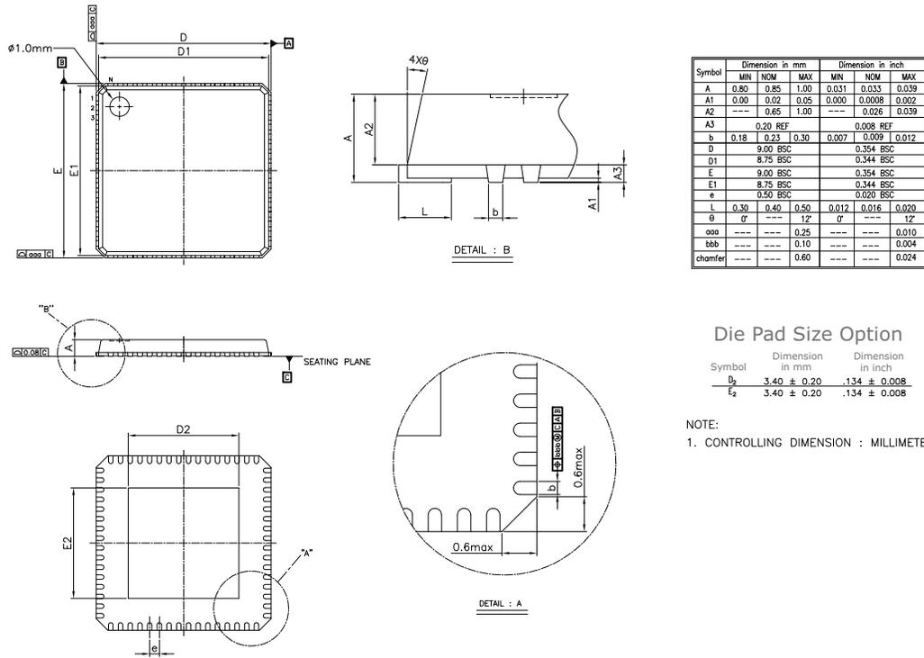
Figure 2-2. I210 QFN 9 x 9 mm Package
