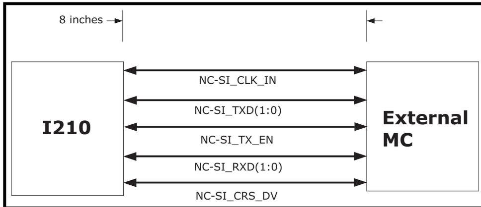
**Figure 12-20. NC-SI Trace Length Requirement for Direct Connect**
