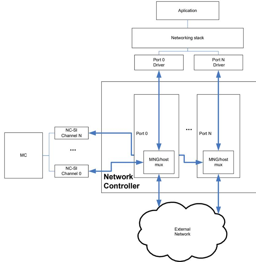
**Figure 10-2. OS-to-MC Diagram**
