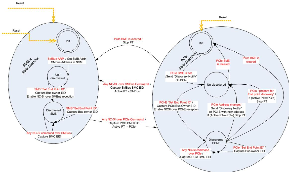
Figure 10-10.MCTP Bus Transition State Machine
