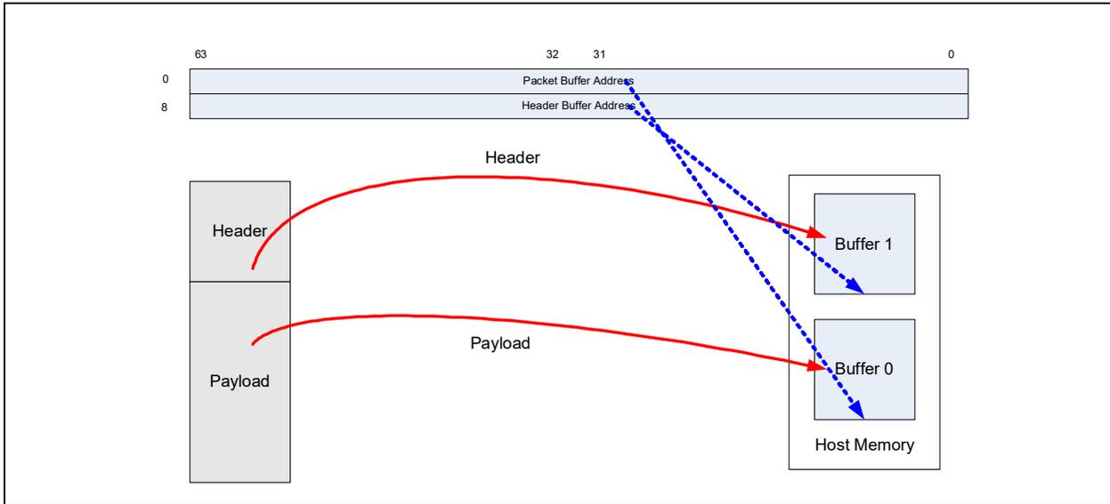
Figure 7-8. Header Splitting
