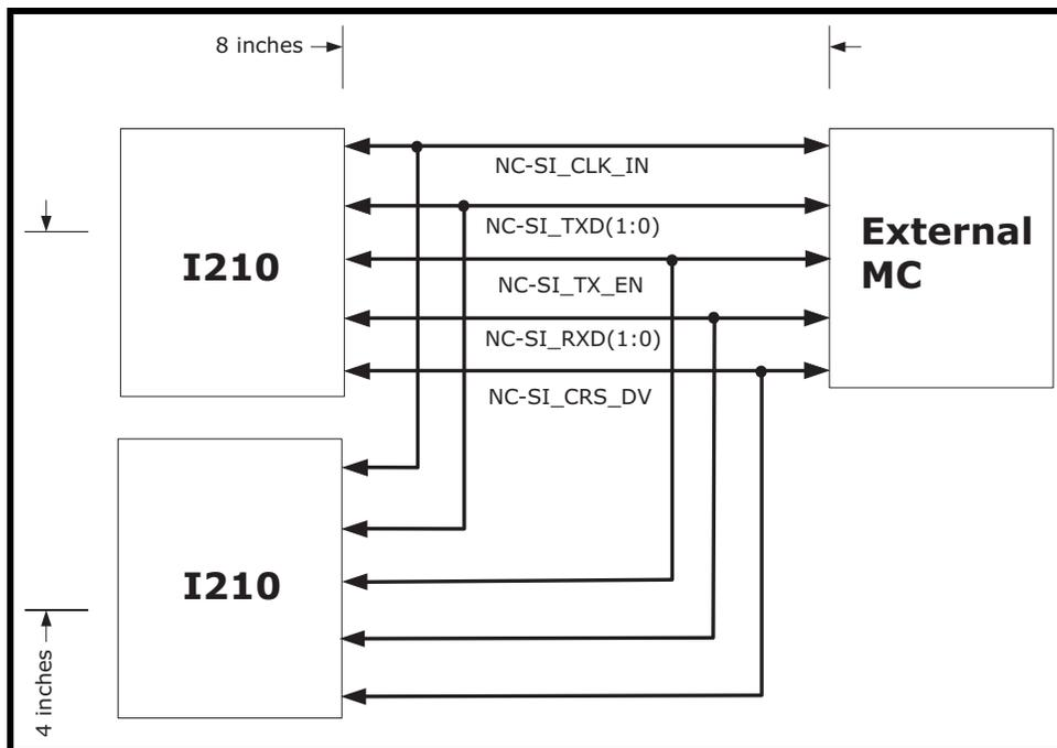
**Figure 12-21. NC-SI Trace Length Requirement for Multi-Drop**
