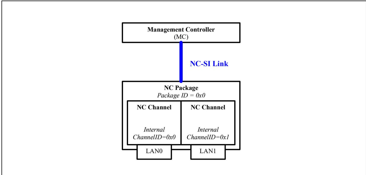
Figure 10-4. Single NC Package, Two NC Channels
