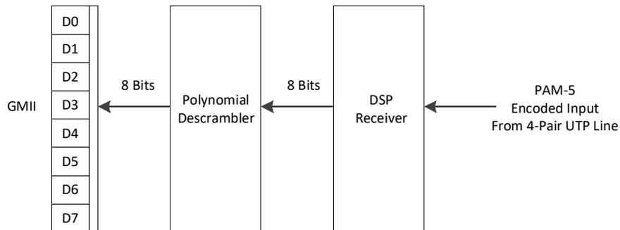
Figure 3-20. Transmit/Receive Flow
