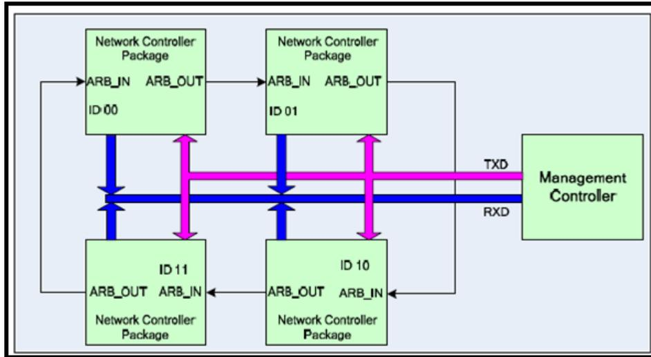
Figure 12-19. NC-SI Connection Requirements - Hardware Arbitration
