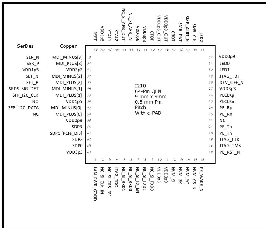
Figure 2-1. I210 64-Pin, 9 x 9 QFN Package With e-Pad
