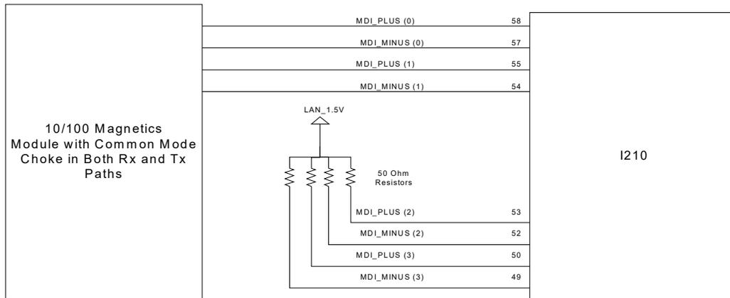
**Figure 12-12. I210 10/100 Mb/s Magnetics Module Connections (With CMC)**
