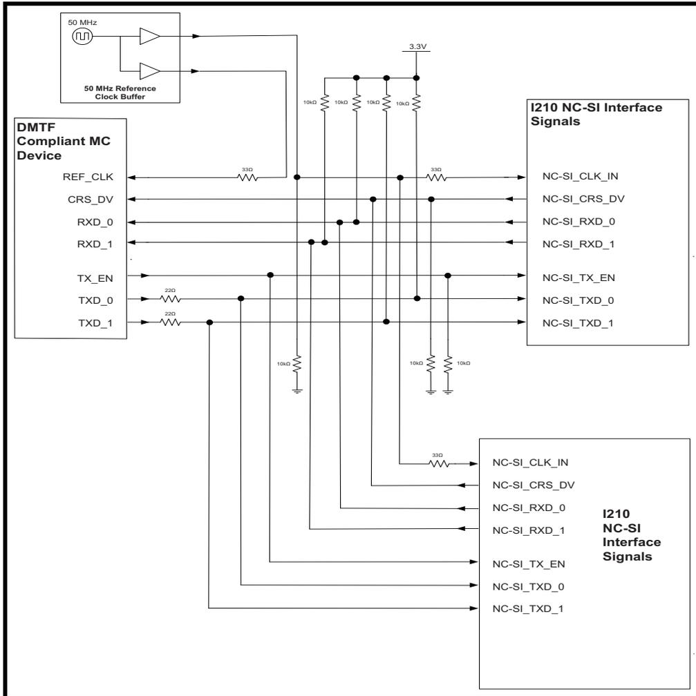
Figure 12-18. NC-SI Connection Requirements - Multi-Drop Configuration
