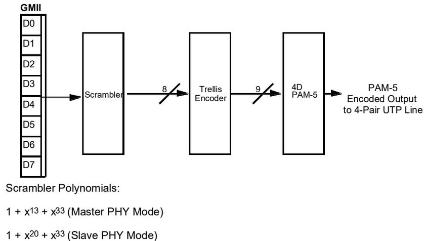
Figure 3-19. 1000BASE-T Transmit Flow And Line Coding Scheme
